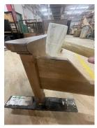
Align the footboard with the side rails, ensuring the slots on the posts align with the hooks on the rails, and repeat the same process. Using a rubber mallet, gently tap the top of each side rail near the post to ensure the hooks are properly seated.
